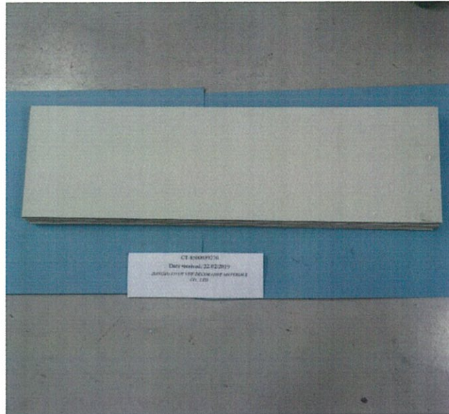
Photo. 1: Fifteen (15) pieces of "Decobond film laminated metal composite panel, 4 mm, PR-A", each of nominal test size of 885mm x 270mm x 3.2mm were received on 22/02/2019.
